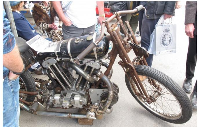
Our road-registered Norton had been in pieces four weeks earlier, had the engine rebuilt, Manx forks and wheels added, and 80 breaking-in miles put on it in the days before the Meet. On Friday the bike completed morning practice and qualifying to get placed in the middle of the field for the Barry Sheene Memorial Trophy races at the weekend. The afternoon was spent sorting out the camshaft drive, then the bike was wheeled out
