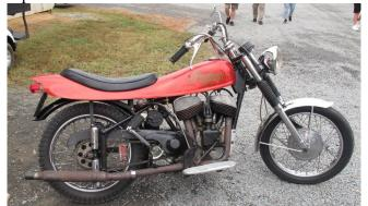
This is one of about 39 built by West Coast dealer Sammy Pierce with an eye-catching metalflake red fiberglass tank/seat over used Scout parts in a 1949 Warrior frame. Custom and cool!
