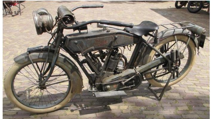
I'm a big fan of these 61 cubic inch (1000 cc) overhead valve V-twins, with both front and rear suspension, and this one looks to be in first paint. Pope turned to making military equipment in WW1, with the motorcycles not reappearing afterwards.
