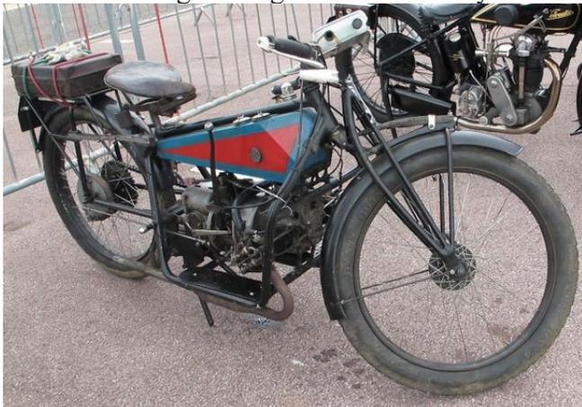
And this 1929 Zenith is a typical British machine fitted with the 750 cc JAP V-twin.
