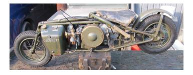
It's a 1942 Welbike, designed in secret at Welwyn in Hertfordshire, and intended to be dropped in a parachute container. The commandos are then supposed to unfold and pin the handlebars and seat in about 15 seconds so it looks like this:
