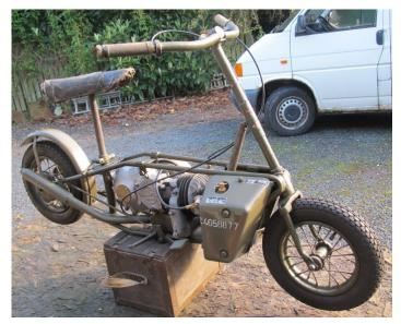
With a push start it is then ridden to the front line on the 98 cc two stroke engine, with about a quart/litre of fuel and then abandoned. About 3,000 were built, with many surplused as pit bikes or farm transport as there is no front brake. If that is not to your taste, how about this 1940 Matchless G80 in original paint?
