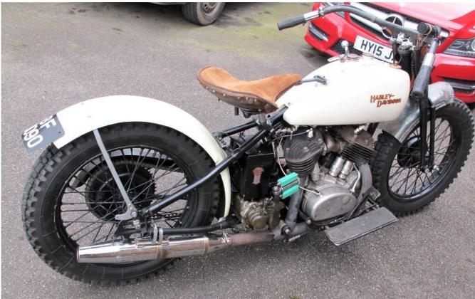
The open pipes were too loud, so I found a pair of 2003 old stock Harley mufflers and put one on. It has a catalytic converter, giving exciting flames out of the back in the early days with a rich mixture.
