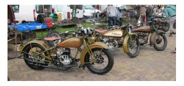
That's a C single side valve of 500 cc, using the same cycle parts as the early small twin, a 350 cc BAH twin port 350 cc overhead valve, and the 1200 cc flat head VL Big Twin. And here's an original paint 1937 knucklehead, said to be the last bike imported into Austria before it became part of the Third Reich:
