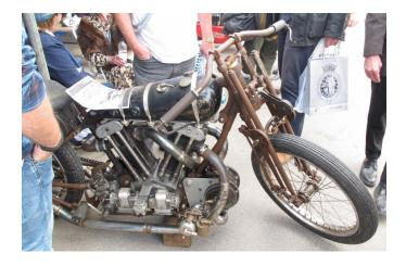
Our road-registered Norton had been in pieces four weeks earlier, had the engine rebuilt, Manx forks and wheels added, and 80 breaking-in miles put on it in the days before the Meet. On Friday the bike completed morning practice and qualifying to get placed in the middle of the field for the Barry Sheene Memorial Trophy races at the weekend. The afternoon was spent sorting out the camshaft drive, then the bike was wheeled out
