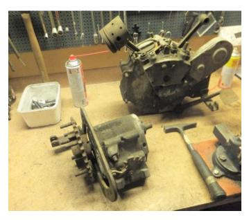
When the engine was split, what was hidden in the crankcase? Well a rusty crank section of eight kilos with an iron piston that weighed 700 grams. All bearings and crank pins had to be newly made, the connecting rods must be aligned and new pistons had to be procured. The engine was sent to "Indian Parts Europe" in Denmark. Everything had to be manufactured according to my parts and it was not cheap but this is the heart of the engine and it was a very nice job I got back.
