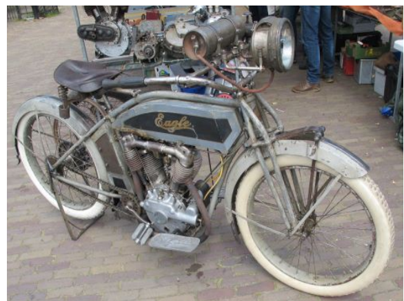
This used the Spacke engine, like the Dayton and Sears, with 1915 being their last year.
