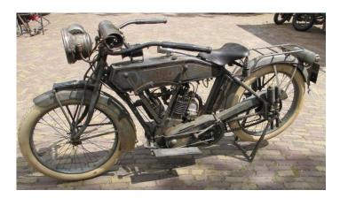
I'm a big fan of these 61 cubic inch (1000 cc) overhead valve V-twins, with both front and rear suspension, and this one looks to be in first paint. Pope turned to making military equipment in WW1, with the motorcycles not reappearing afterwards.
