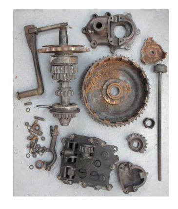
It is a Harley VL reverse gearbox rescued from the fire at that Austrian museum, which was hot enough to melt the aluminium case. So an easy fix, right? A week in a bucket of diesel, pull it apart, bead blast the parts, re-harden the gears and shafts, find another case, with the result then probably costing only slightly more than buying a restored one...
